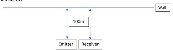
Method 2; This method uses a spectrum analysis microphone deployed at distance x from a loudspeaker emitting pink noise. The transfer function of the sound will give us a time in milliseconds between the sound being generated and being measured.
